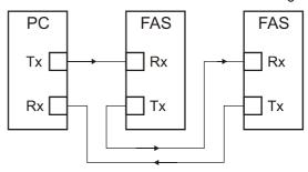
Networking with an RS 232 ring is supported by FDS Tool.
