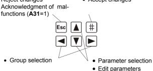
To program, press the # key (Enter). The menu consists of several groups which are identified with the letters A, B, C and so on. Select the groups with the arrow keys (i.e., ◀ and ). Press the # key again to access the parameters of the selected group.
