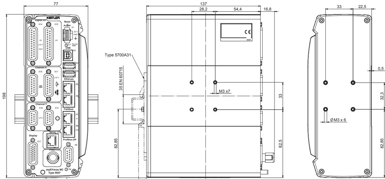
Note: Observe minimum spacing of >10 mm between the MEM's!
