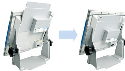
The DIM Cable Extender is inserted at the rear portion of the display. The DIM Cable Extender is supplied with 24 V of power (the display is then supplied by the DIM Cable Extender). The DIM Cable Extender is connected to one or several maXYmos units via an Ethernet cable.
