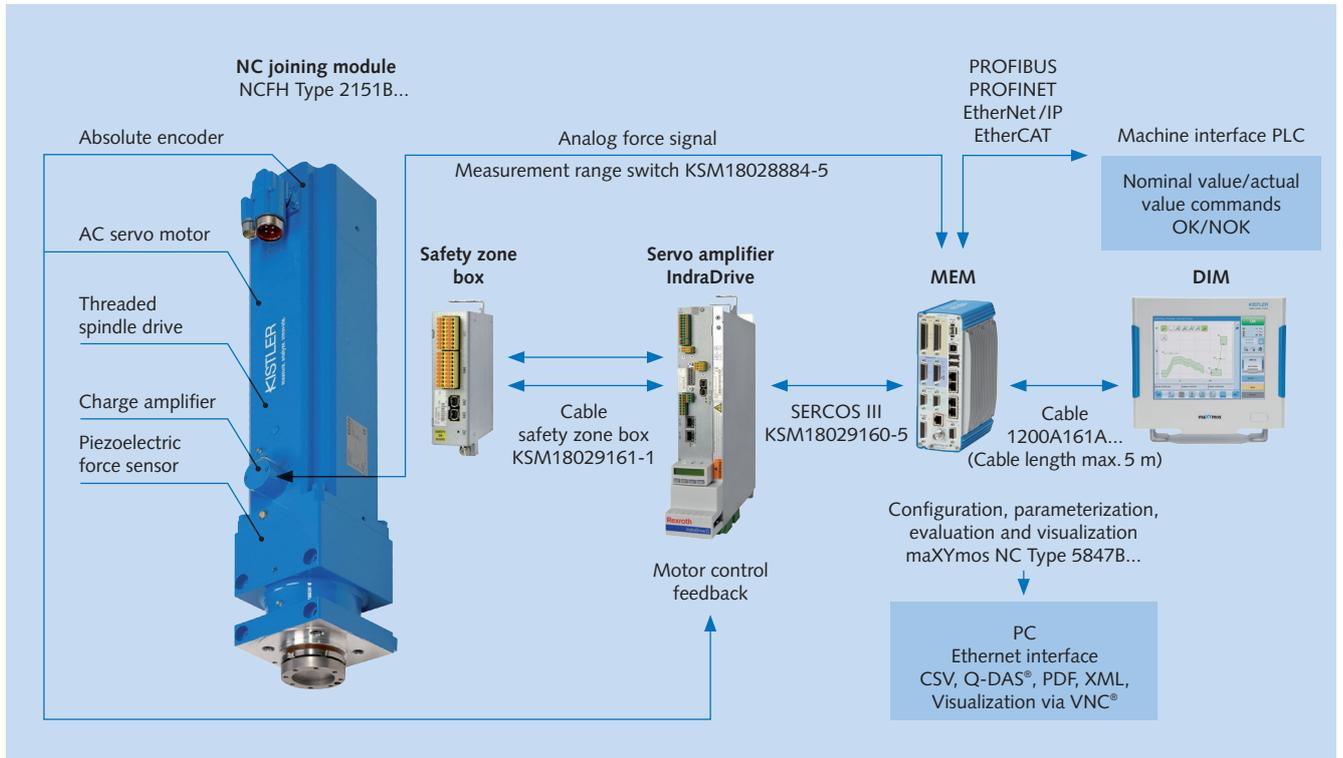
Functional principle of an NC joining system using the NC joining module NCFH Type 2151B... and maXYmos NC Type 5847B...
