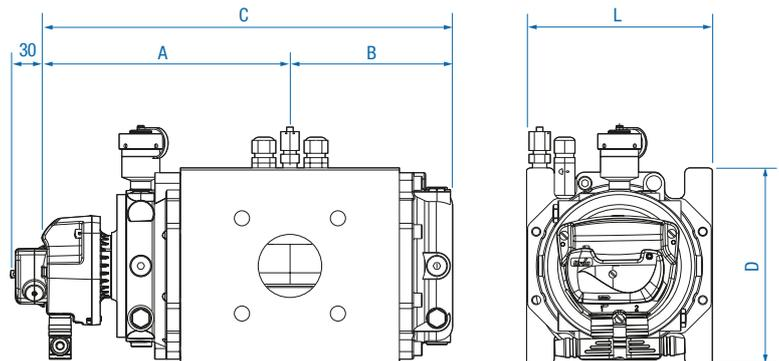
Delta DN80 G100 3xDN in Ductile iron equipped with Cyble sensor
