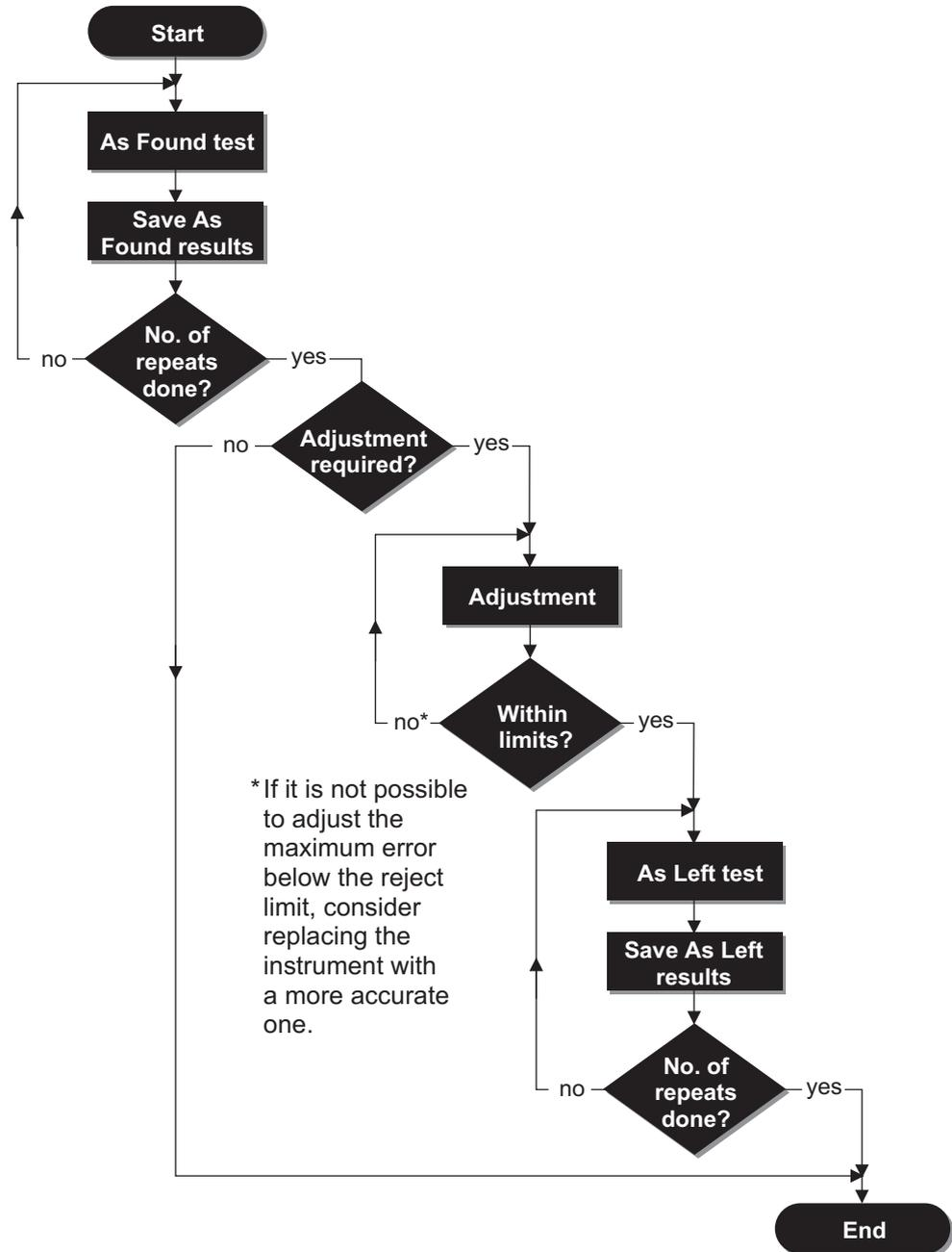
The picture gives a general view of the phases in a typical calibration procedure.
