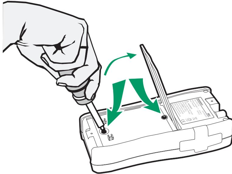
1. Turn MC2 upside down (the display facing the table top) and lift the support.
