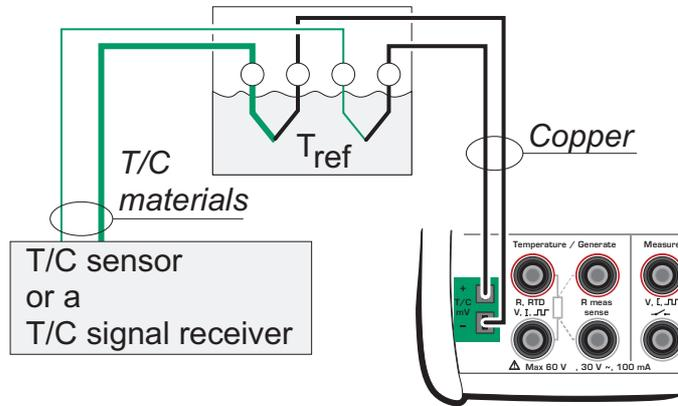
Connection when measuring/simulating thermovoltages using a compensation box and either of the following Reference Junction compensation methods:
