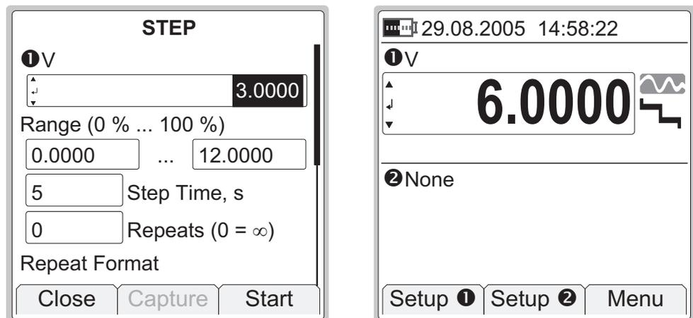
Start stepping by selecting the **F3/Start** Function Key in the configuration window. To stop a stepping that is in progress, open the stepping configuration window and press **F1/Stop Step** Function Key.
