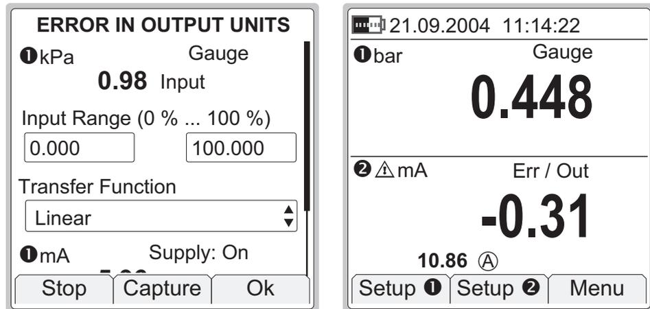
When Error In Output Units display is active, the warning triangle is shown together with the input unit and the text "**Err / Out**" is shown above the Error value.
