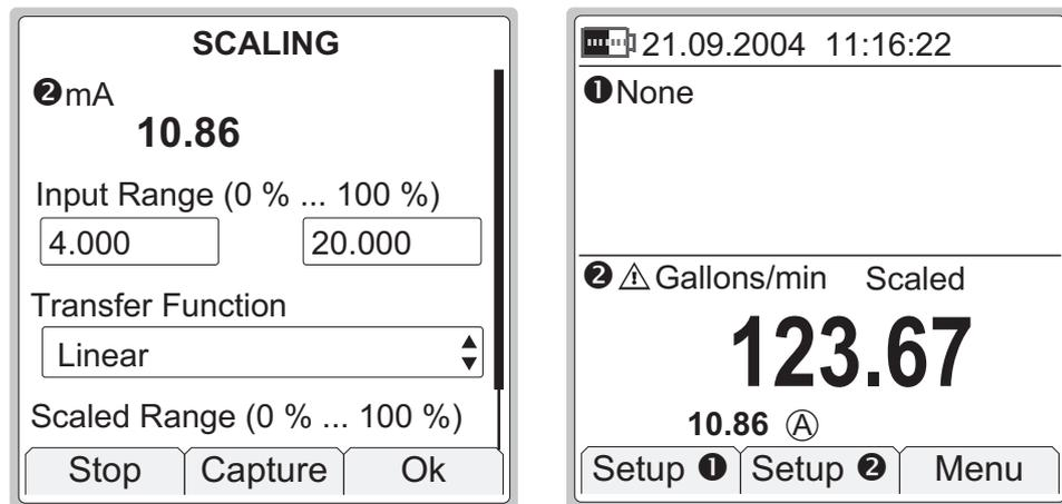
When Scaling display is active, the entered unit (or the text "**scaled unit**" if the unit was not entered) is displayed after the warning triangle and the text "**Scaled**" is shown above the Scaled value.
