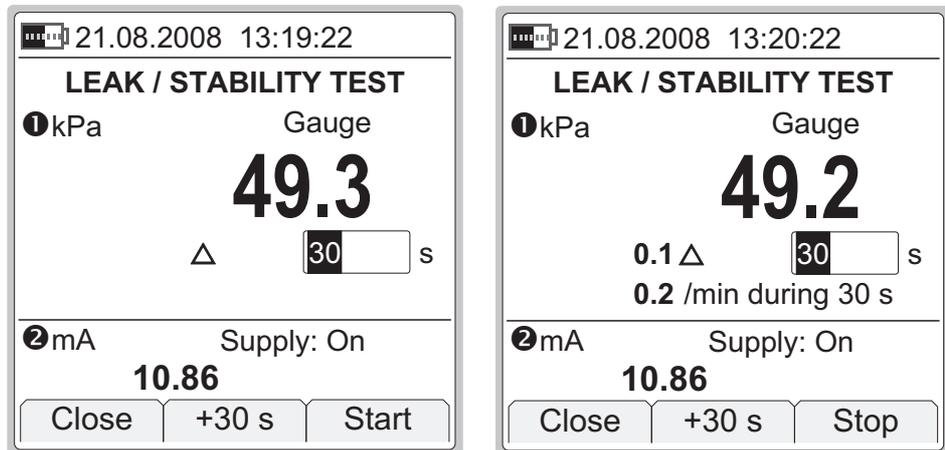
To start the test, first check the test time to be used. Either accept the default value or enter another time period in seconds. Entering zero as the test time means the test will continue until manually stopped. Select **F1/Start** and see how the test advances.
