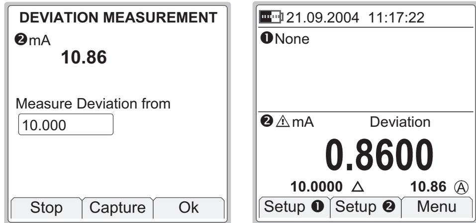
When Deviation measurement is active, text "**Deviation**" is shown above the Deviation value.
