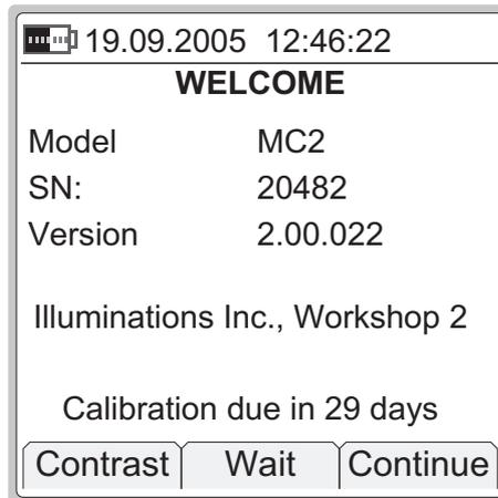
If you want to view the calibrator information for a longer period, press the **F2/Wait** Function Key. Then the calibrator information is visible until you press the **F3/Continue** Function Key.
