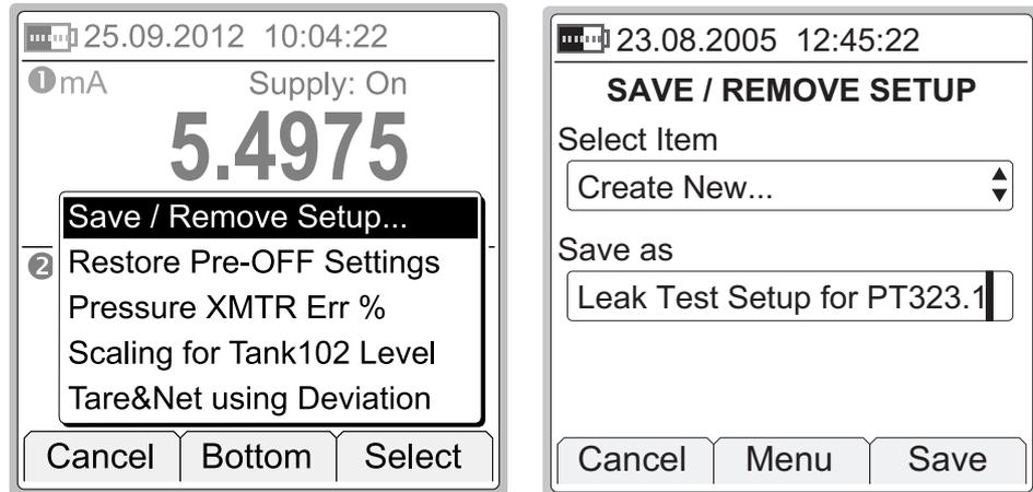
In the leftmost picture above, three User Setups are already saved. Selecting Save / Remove Setup option opens the **SAVE / REMOVE SETUP** window allowing you to save the current settings for window ❶ and window ❷ (see rightmost picture).
