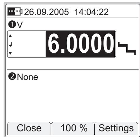
Start manual stepping by selecting the **F3/Start** Function Key in the configuration window. To stop it, press **F1/Close** Function Key (in Basic Mode).
