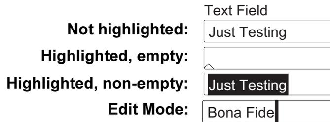
Beside the Enter key (↵), all Numeric keys set the highlighted Text field to edit mode. The Enter key leaves the previous text available for editing and the Numeric keys replace the old text.
