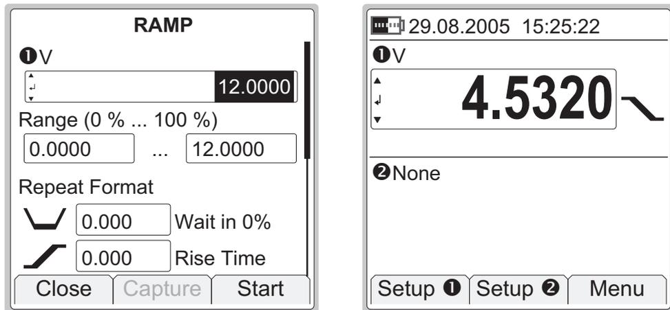
Start ramping by selecting the **F3/Start** Function Key in the configuration window. To stop a ramp that is in progress, open the ramping configuration window and press **F3/Stop** Function Key.
