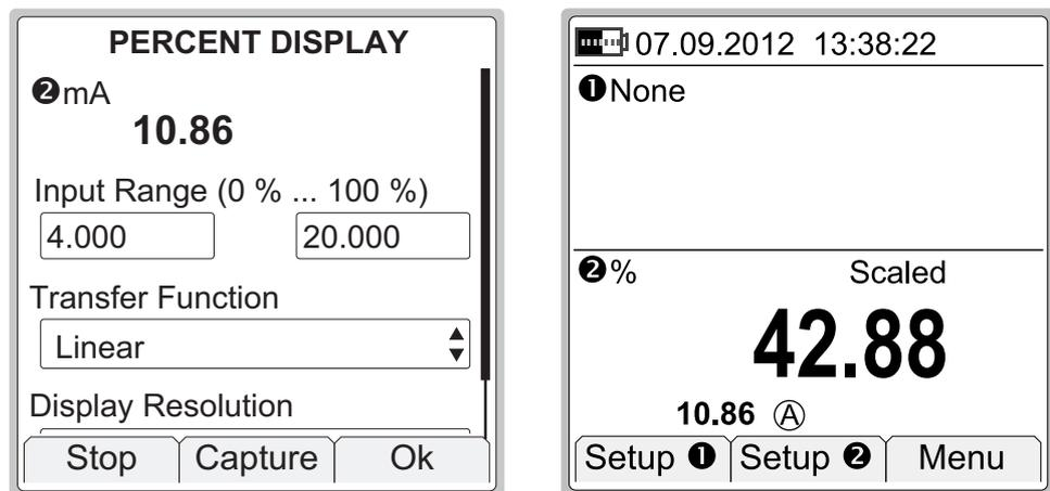
When Percentage display is active, the letter "%" is displayed after the warning triangle and the text "**Scaled**" is shown above the Percentage value.
