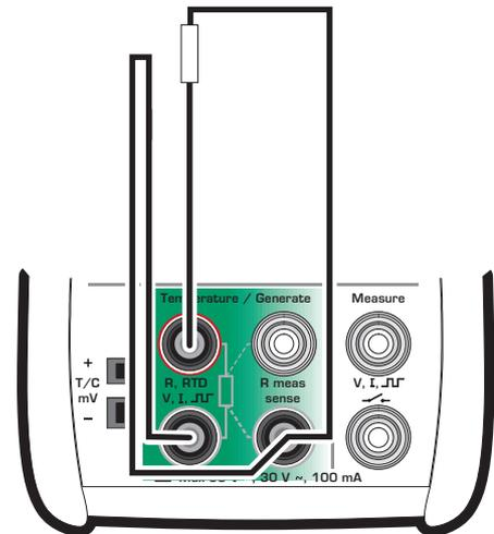
If the compensation loop and the connection wires of the resistor are identical, MC2 can compensate for the resistance of the connection wires.
