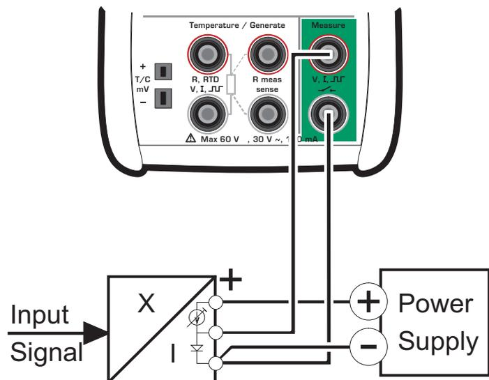
MC2 parallels the test diode of the transmitter and measures the externally supplied output current of the transmitter.
