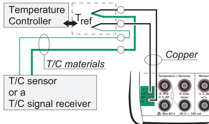
Connection when measuring/simulating thermovoltages using a fixed temperature and either of the following Reference Junction compensation methods:
