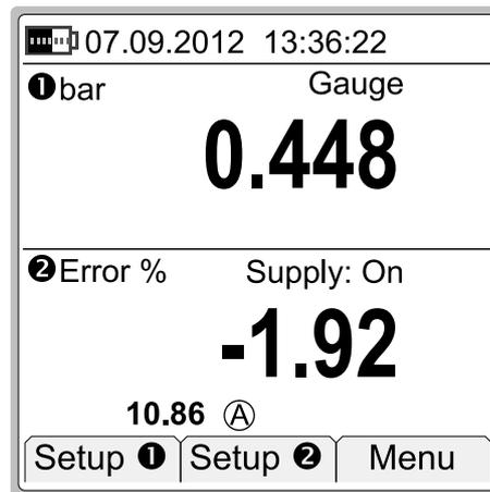
The picture above is an example where a pressure transmitter is calibrated using error percentage display mode for the output current. The additional info row displays the actual output current of the instrument. Another useful method, especially while adjusting the instrument, is displaying the error bar graph in the additional info row.
