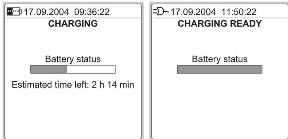
The charging time depends on calibrator's current consumption (backlight, mA sourcing etc.). With no extra load, the charging time is approx. 5 hours.
