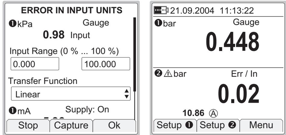
When Error In Input Units display is active, the warning triangle is shown together with the input unit and the text "**Err / In**" is shown above the Error value.
