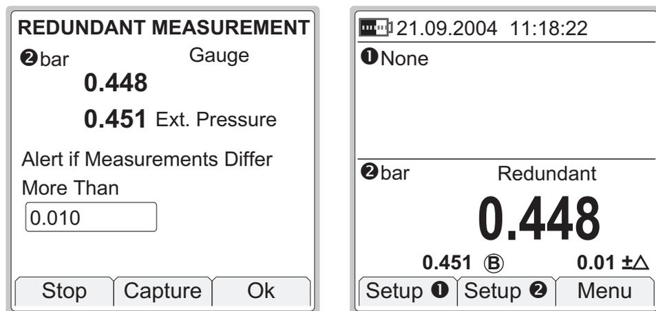
When Redundant measurement is active, text "**Redundant**" is shown above the main measurement value.
