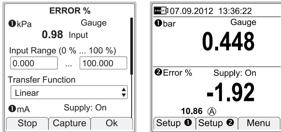
When Error Percentage display is active, the words "**Error %**" is displayed after the warning triangle.
