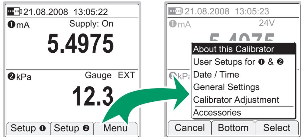
The pair of screenshots above is an example of an opening menu. This one opens from Basic Mode when F3 Function Key is pressed.
