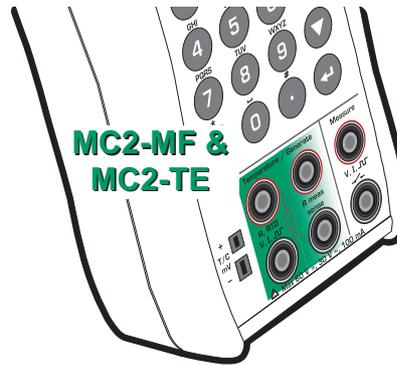
The two leftmost terminals are used in 2-wire systems. MC2 automatically checks the connection and displays the found wiring system (2-wire, 3-wire or 4-wire) in the upper right corner of the measuring window. For more information concerning wiring options, see **Resistance and RTD Measurement, Connections** on page 116.
